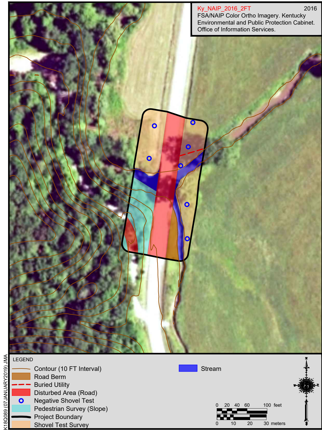
Figure 6. KY 191 bridge (119B00001N) over Lacey Creek (Item No. 10-10009.00) in Wolfe County showing shovel test locations on an aerial map.
